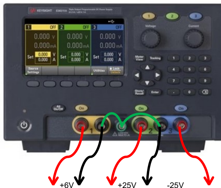
Figure 3 – DC Power Supply Connections
